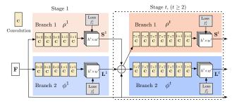
Figure 3. Architecture of the two-branch multi-stage CNN. Each stage in the first branch predicts confidence maps  $\mathbf{S}^t$ , and each stage in the second branch predicts PAFs  $\mathbf{L}^t$ . After each stage, the predictions from the two branches, along with the image features, are concatenated for next stage.
